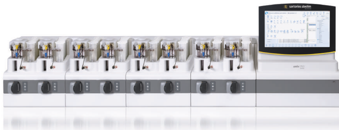
Figure 2: The ambr® 250 modular bioreactor system can now even be used for cell and gene therapy applications.
